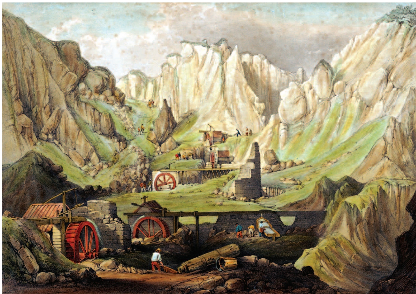
Figure 6. Lithograph of 'Carclaze Mine' thought to have been published by Philip Mitchell in 1841 (reproduced by kind permission of Royal Cornwall Museum, Royal Institution of Cornwall), although it may depict a scene from earlier. Probably looking east; five waterwheels can be seen which are powering stamps, a discarded stamps barrel is seen in the right foreground and a sloping table on the right is being used to recover coarse tin. The movement of material in the pit can be seen to be by wheelbarrow.
